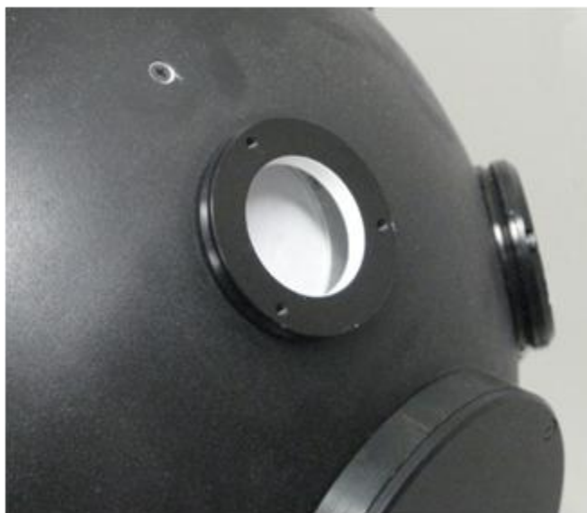
Figure 3-24. View of the opening in the sphere for the primary lamp, showing the internal baffle used to create a more uniform field.
