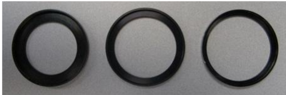
Figure 3-20. Three mounting rings used to attach the neutral density filters to the lenses (one for each lens).
