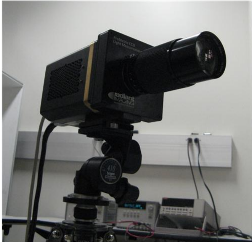
Figure 3-14. Digital Imaging Photometer mounted on a tripod with a zoom lens
