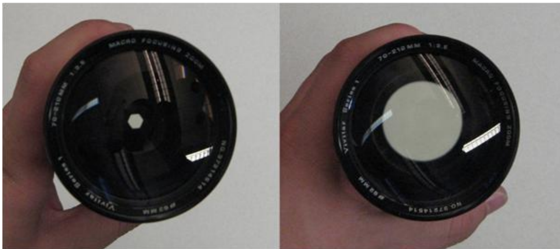
Figure 3-18. Images of Promaster zoom lens showing changes in aperture based on different f-stops. Left is f/22 and right is f/3.5 .
